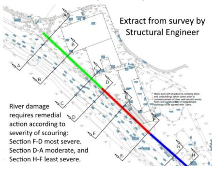
D-A: Extent of existing rubble stone wall to be re-pointed and missing stonework replaced.
